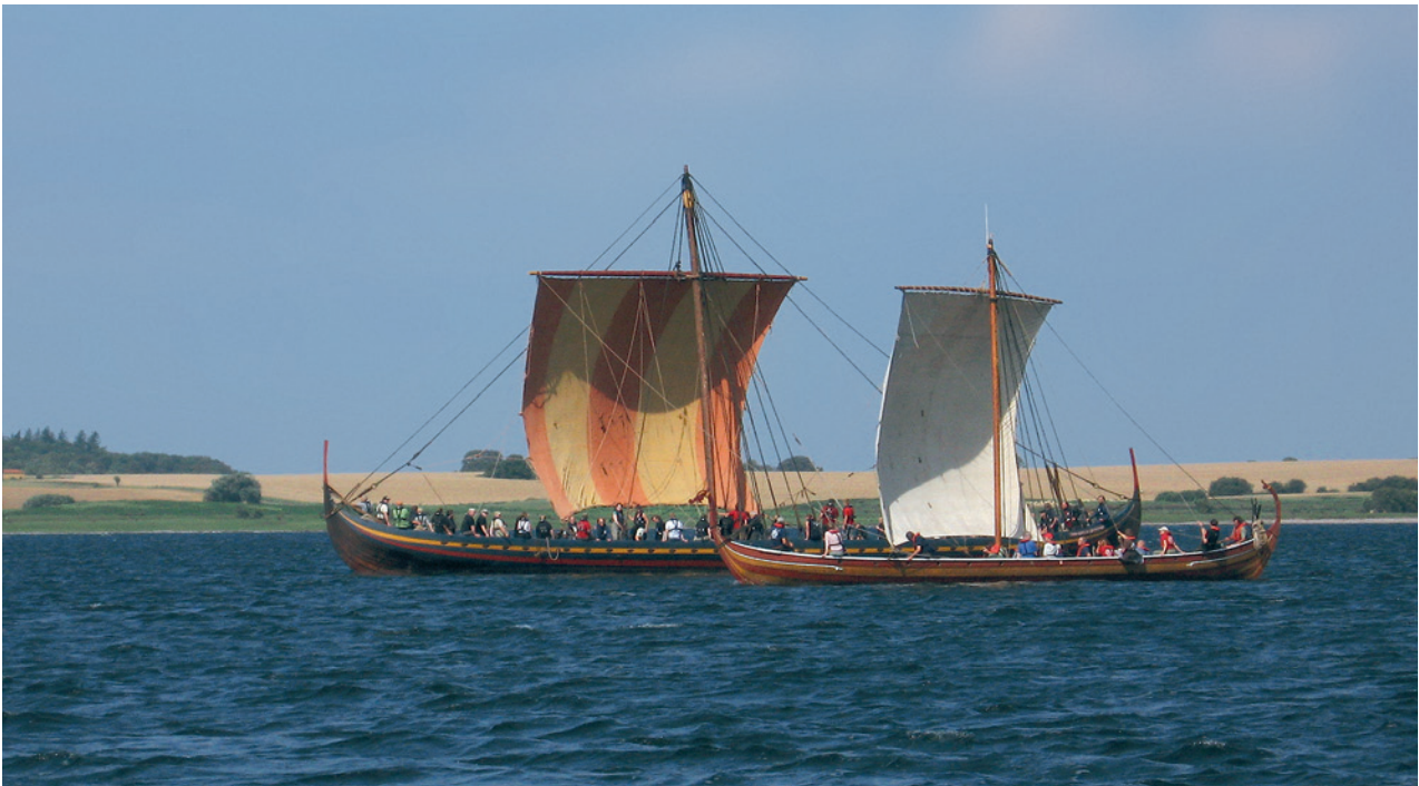
Fig. 8. The Viking Ship Museum's full-scale replicas of the warships Skuldelev 2 and 5, respectively The Sea Stallion of Glendalough (2004) and Helge Ask (1990), in Roskilde Fjord, August 2009. The Sea Stallion (furthest away) has a reefed sail due to the force of the wind. This means that its sail is lower than at full sail.
